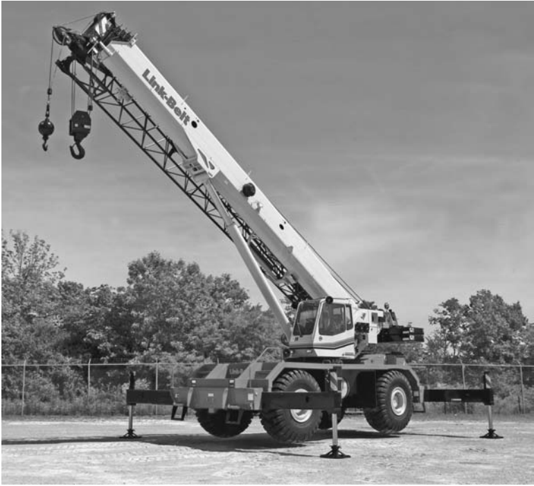
FIGURE 1.2 Link-Belt model RTC-8090 Series II rough terrain crane. Note the two wire ropes each leading from a winding drum over the upper surface of the boom to a deflector sheave at the boom tip. One rope continues to the fixed upper block and thence to the load block, while the other runs over a second deflector sheave to the auxiliary hook and ball. ( Link-Belt Construction Equipment Company. )
