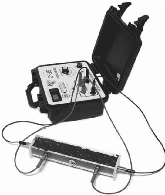
FIGURE 5.13 Soil box and resistivity equipment. (Courtesy of Tinker & Rasor)
